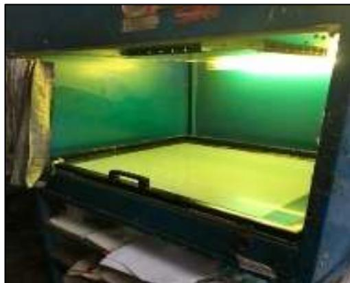
Gambar 3.3 *Plate making* film
